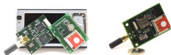
Figure 1. Split- and single-board sensor board designs.
