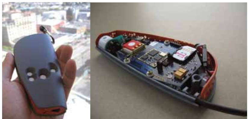
Figure 2: Handheld Monitor Design and Enclosure Source: Photo by Mazzarello Media and Arts 2009
